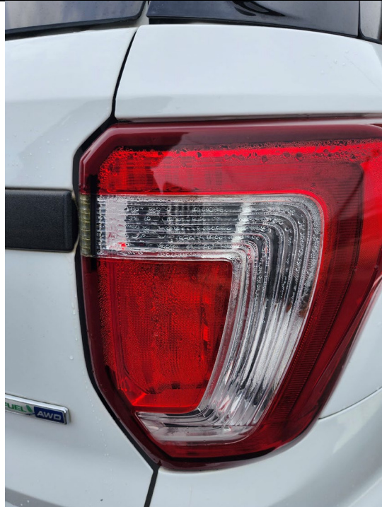
Vehicle 161: Passenger side rear taillight has water and moisture inside
