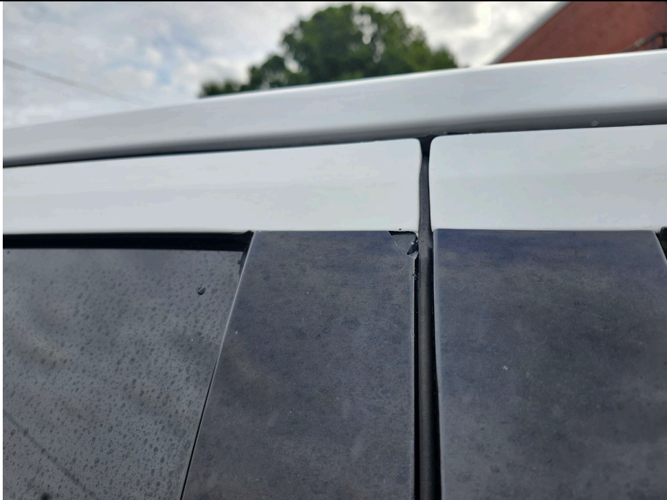
Vehicle 161: Passenger side rear door molding is broken
