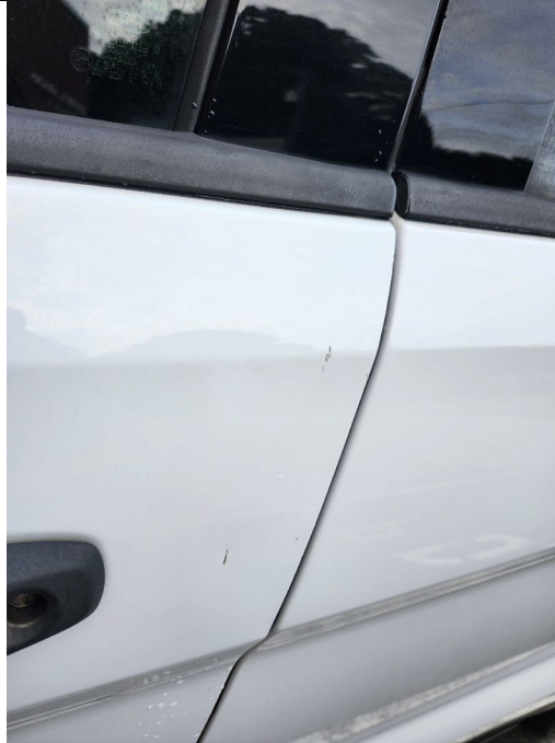
Vehicle 161: Driver's door has several small dents
