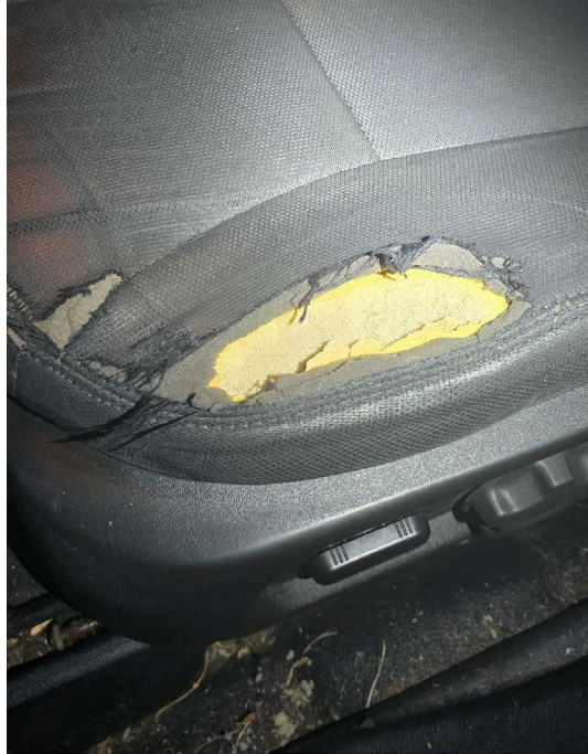
Vehicle 173: Driver seat has an approximately 2” hole in seat with metal exposed
