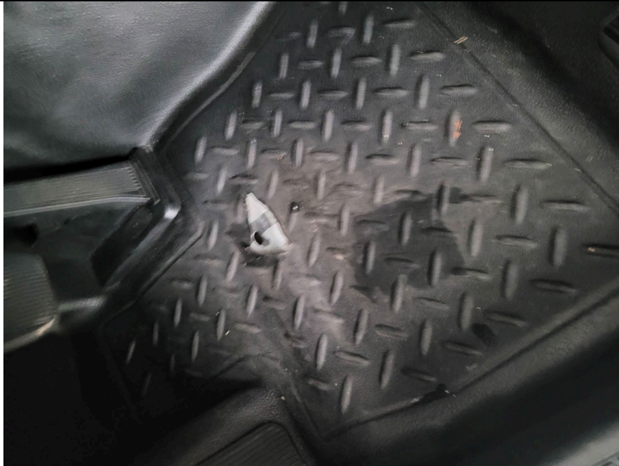
Vehicle 201: Hole in floor on the driver's side where the rubber mat is worn
