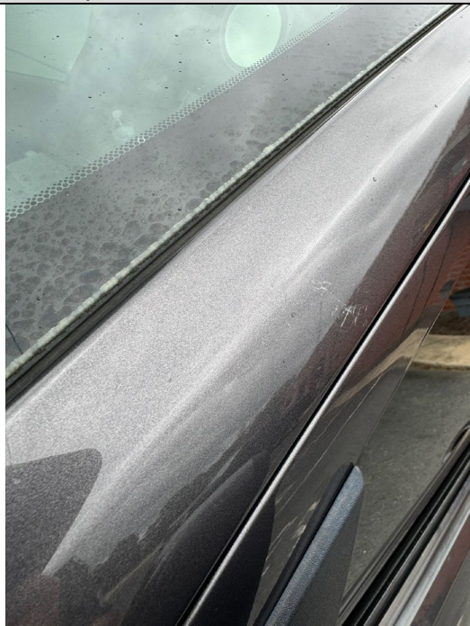
Vehicle 191: Paint scratch on A post
