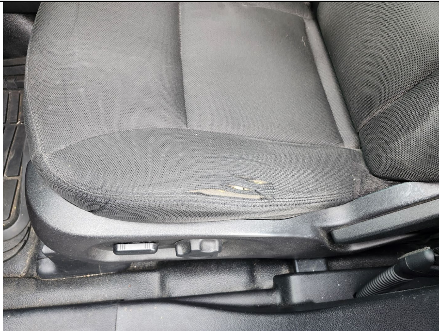
Vehicle 161: Driver's seat is starting to come apart and is showing wear
